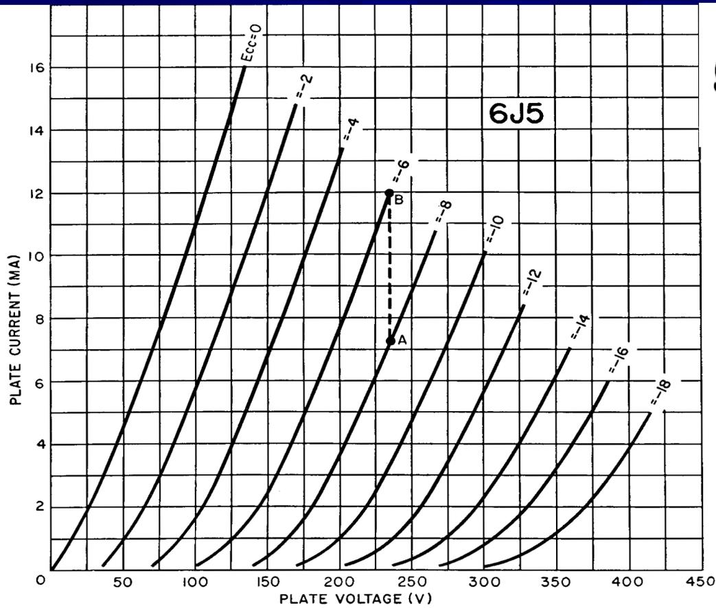
Figure 58. Plate family of curves used to determine transconductance of 6J5 triode.
