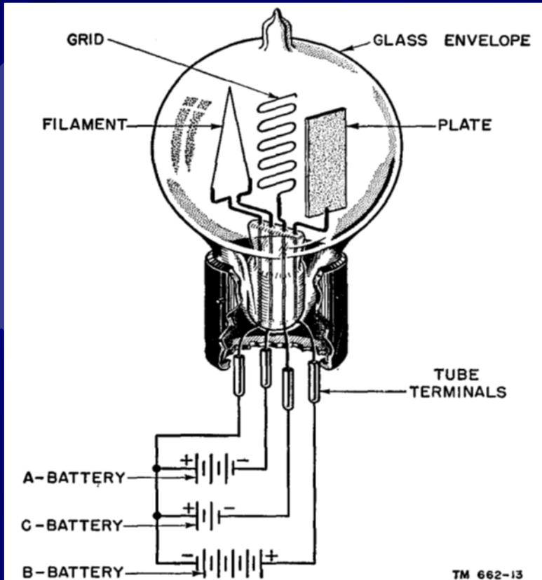
Figure 4. Construction of DeForest's three-element tube, or triode.
